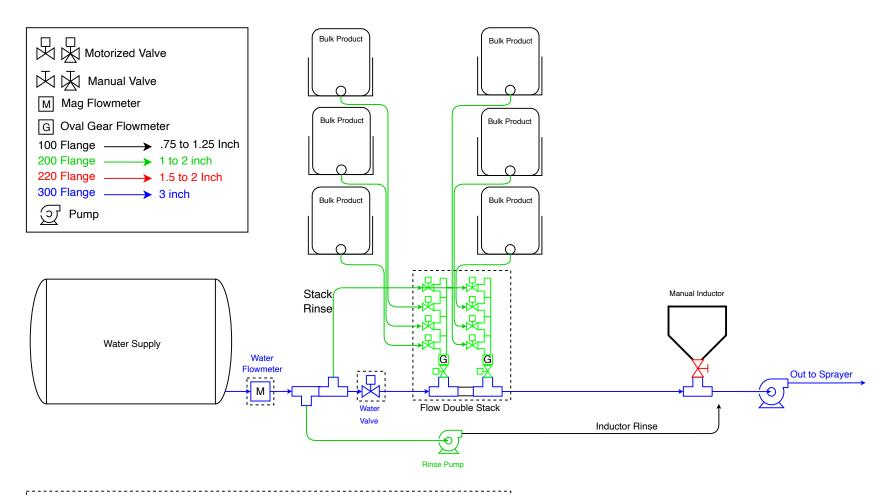
Mixmate six input Double Stack. All chemicals are measured with gear type flowmeters. Up to two bulk chemicals will be measured simultaneously while using the inductor. Consult your dealer for variations to this configuration.
