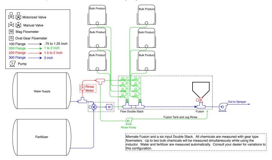
The Rinse Pump supplies pressurized rinse water to the Inductor and jug rinse. Kits: K1a, K3, K18, 2-K46, K34, K53, K33
