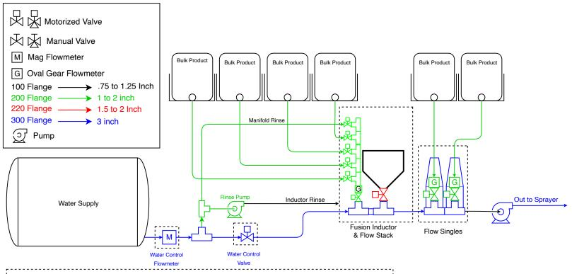
Mixmate Fusion with a three input stack. All bulk chemicals are measured with a gear type flowmeter. Three bulk chemicals will be measured simultaneously while using the inductor. A Stack add-on valve and two Flow Singles complete this six input system. Consult your dealer for variations to this configuration.
