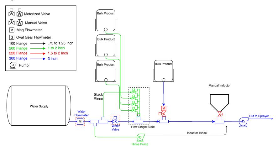
Mixmate three input Single Stack. All chemicals in the stack are measured with gear type flowmeter. An input with a two inch magmeter and valve will measure at the same time as the Flow Stack. This configuration is good for fertilizers and thick chemical that can be measured with a magmeter. Consult your dealer for variations to this configuration.
