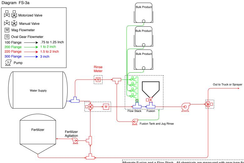
Mixmate Fusion and a Flow Stack. All chemicals are measured with gear type flowmeters. Dry fertilizers can be premixed and used as part of a blend. Water and fertilizer are measured automatically. Consult your dealer for variations to this configuration. Does not include electric pump control or a tablet.
